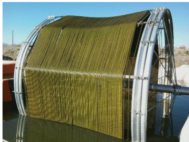
(a) Rotating microalgae biofilm device Hans C. Bernstein et al. 2014
